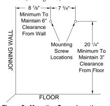
Figure 5 - Mounting Screw Locations
